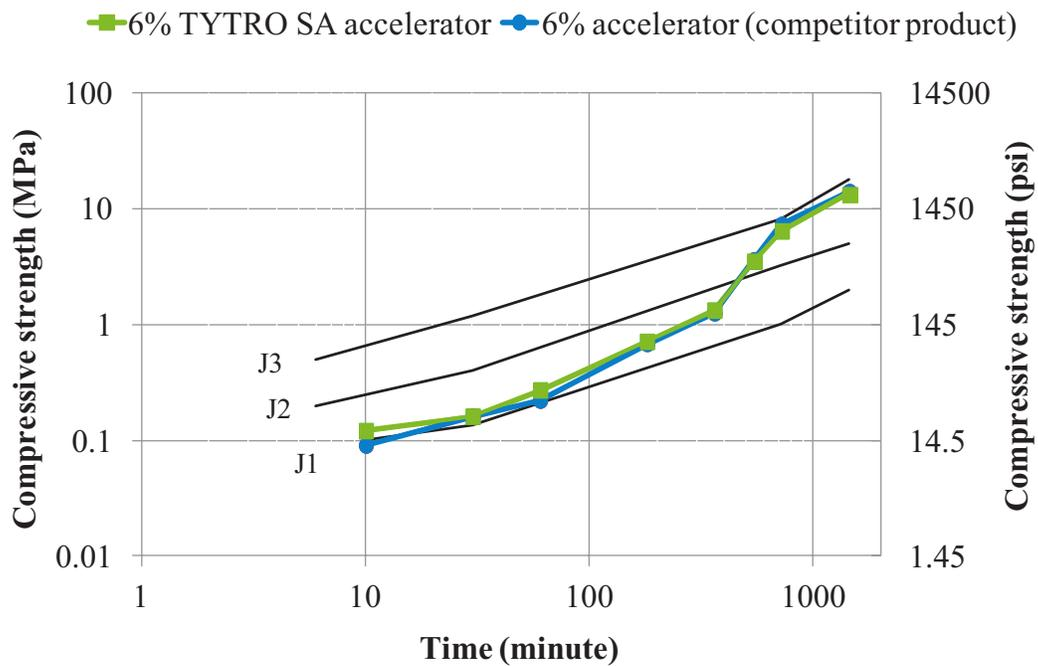
Figure 1. The performance comparison of TYTRO® SA accelerator and a competitor product.
