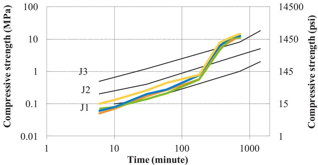
Figure 12. The performance assessment of TYTRO® shotcrete system based on J curves.
