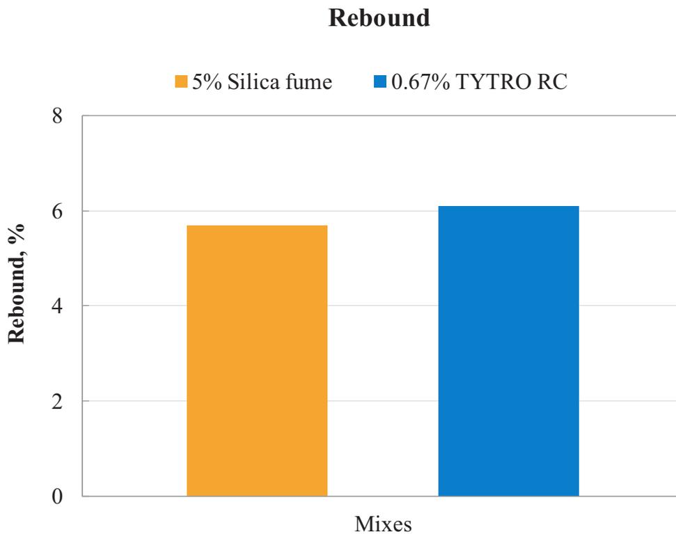
**Figure 9. The effect of TYTRO® RC on rebound.**
