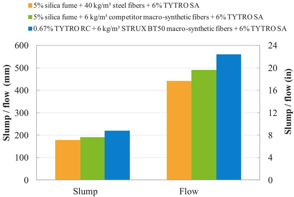
Figure 7. The effect of TYTRO<sup>®</sup> RC and STRUX<sup>®</sup> BT50 macro-synthetic fibers on slump and slump flow at 60 minutes.
