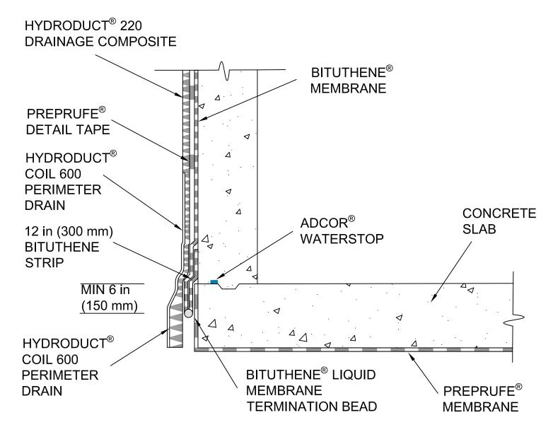
NOTE - GCP MAY REQUIRE AN ALTERNATE GCP WATERSTOP BASED ON DESIGN CONDITIONS
