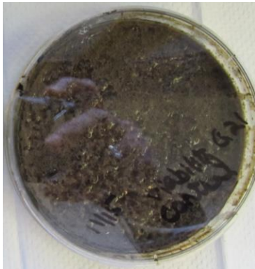
Fig2: Spores Viability control - heavy fungal growth © Accugen labs
