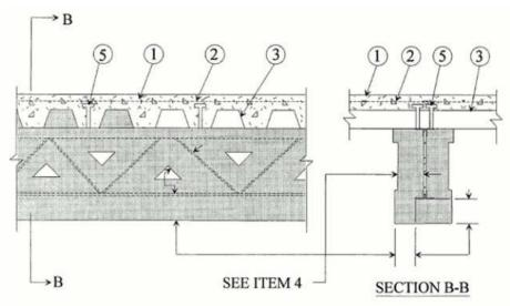
1. **Supports** — W8 x 28 or alternate (per Section IV.6 in the front of the Fire Resistance Directory) steel beam or min 10K1 steel joists when joist substitution applied.
