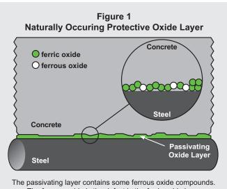
The passivating layer contains some ferrous oxide compounds. The ferrous oxide is the defect in the ferric oxide layer that allows chloride to initiate corrosion. The alkaline environment causes the ferrous ions to become ferric ions (Fe<sup>+++</sup>), according to the reaction:
