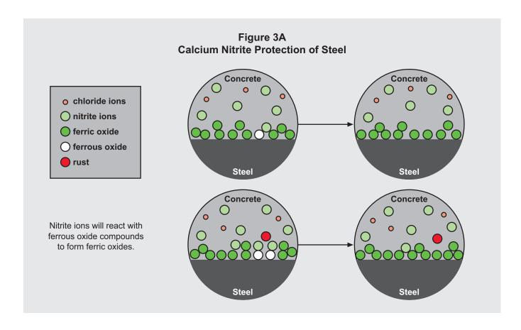
defects are surrounded by nitrite ions, and less likely to be exposed to chloride ion attack.
