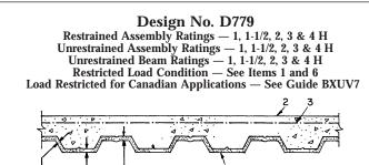
1. Supports — W8 x 28 or alternate (per Section IV.6 in the front of the Fire Resistance Directory) steel beam or min 8K1 steel joists when joist substitution applied.
