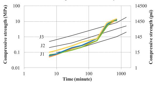
Figure 12. The performance assessment of TYTRO® shotcrete system based on J curves.
