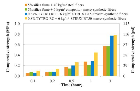
Figure 10. The effect of TYTRO® shotcrete system on very early age strength development up to 3 hours.
