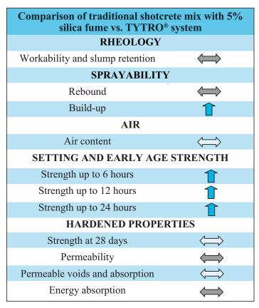
Table 5. Performance comparison of silica fume vs. TYTRO® shotcrete system
