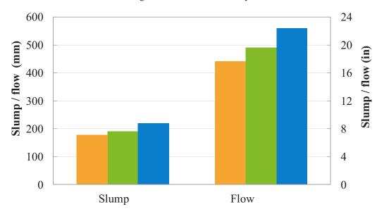
Figure 7. The effect of TYTRO $^{\otimes}$  RC and STRUX $^{\otimes}$  BT50 macro-synthetic fibers on slump and slump flow at 60 minutes.
