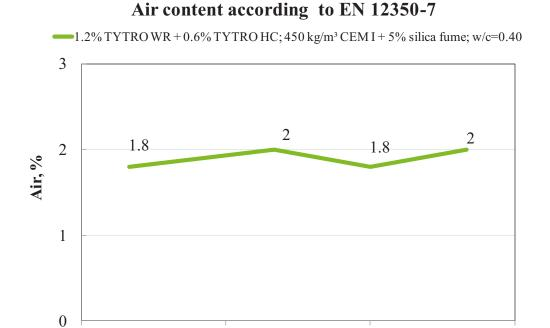
Figure 4. The synergetic benefit of TYTRO® WR and TYTRO® HC combination on air content.
