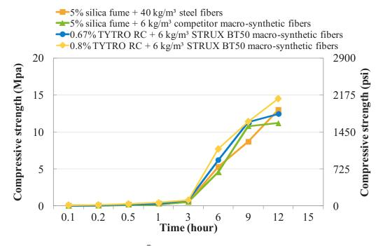
Figure 11. The effect of TYTRO® shotcrete system on early age strength development between 6 to 12 hours.
