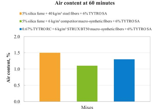
Figure 8. The effect of TYTRO® RC and STRUX® BT50 macro-synthetic fibers on air content.
