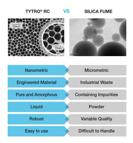
Figure 5. The comparison of properties between silica fume and TYTRO® RC
