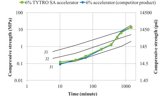
Figure 1. The performance comparison of TYTRO® SA accelerator and a competitor product.
