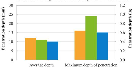
Figure 14. The effect of TYTRO® shotcrete system on permeability at 28 days.
