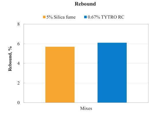
Figure 9. The effect of TYTRO® RC on rebound.
