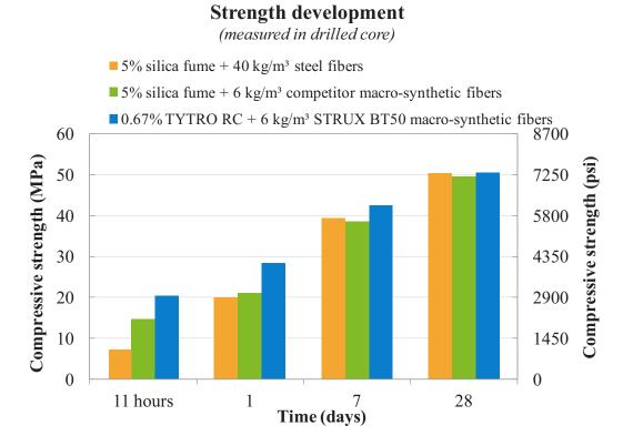
Figure 13. The effect of TYTRO® shotcrete system on strength development up to 28 days.
