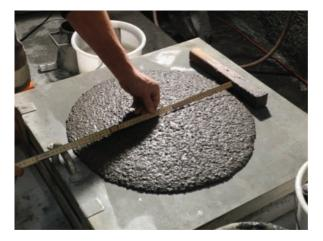
Figure 6. Testing slump and slump flow as an indicator of workability.
