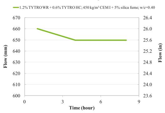
Figure 2. The synergetic benefit of TYTRO® WR and TYTRO® HC combination on flow.
