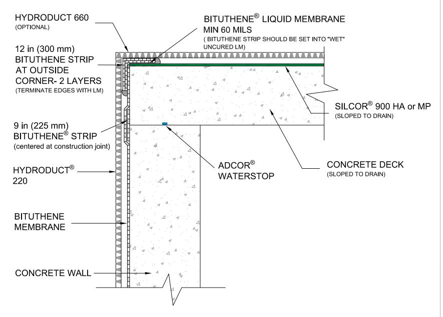
NOTE - GCP MAY REQUIRE AN ALTERNATE GCP WATERSTOP BASED ON DESIGN CONDITIONS
