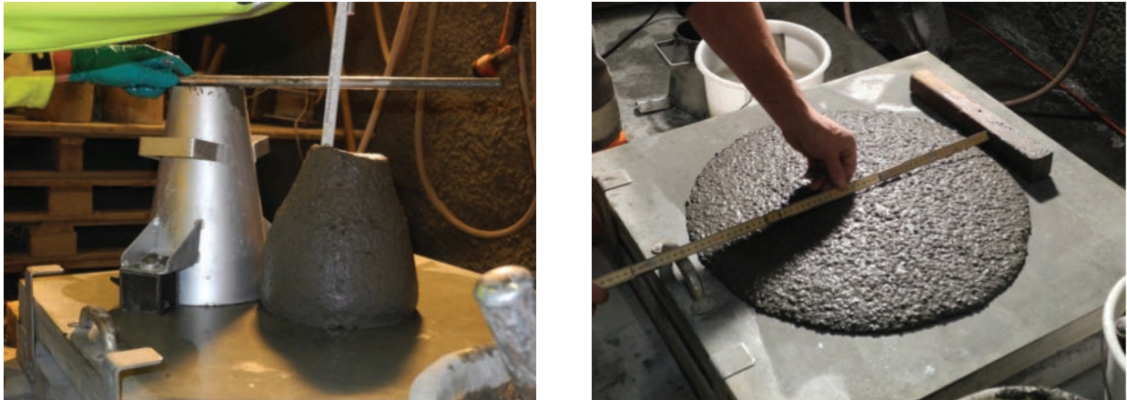
Figure 6. Testing slump and slump flow as an indicator of workability.
