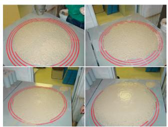
For starters, a plant should develop mix designs for both high flow and low flow applications. Generally, better form finishes are achieved with concrete that has a higher slump flow and lower viscosity. Consult with your GCP representative to decide on admixtures and dosages. Not all HRWR admixtures are created equal and may have different interactions with cement. If one HRWR doesn't work as planned, another may be perfect.
