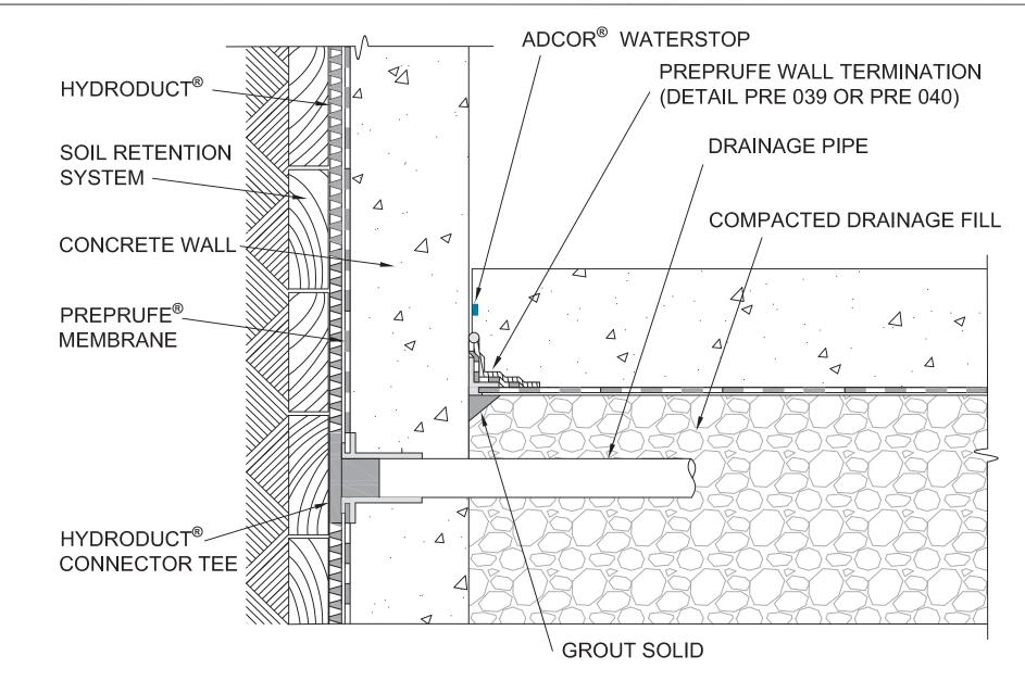
NOTE: - INTENDED FOR PROJECTS WITH PERMANENT DEWATERING OR NON-HYDROSTATIC CONDITIONS
