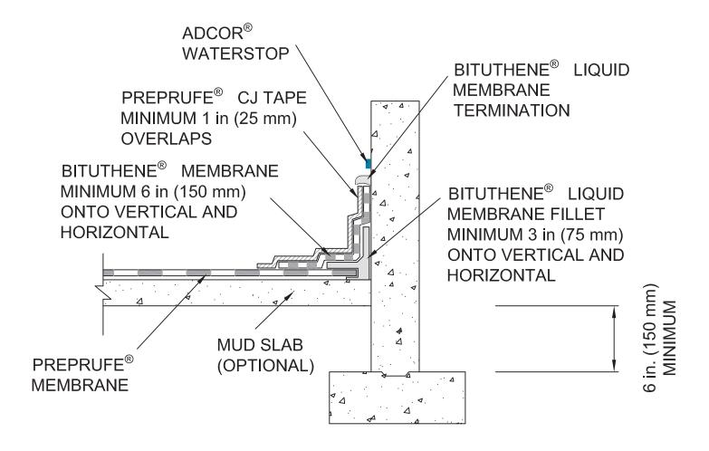
NOTES - IF A MUDSLAB IS NOT USED, THE SUBSTRATE TO ACCEPT THE BITUTHENE LIQUID MEMBRANE MUST BE GROUTED SOLID TO PROVIDE AN ACCEPTABLE SUBSTRATE FOR THE LIQUID MEMBRANE
