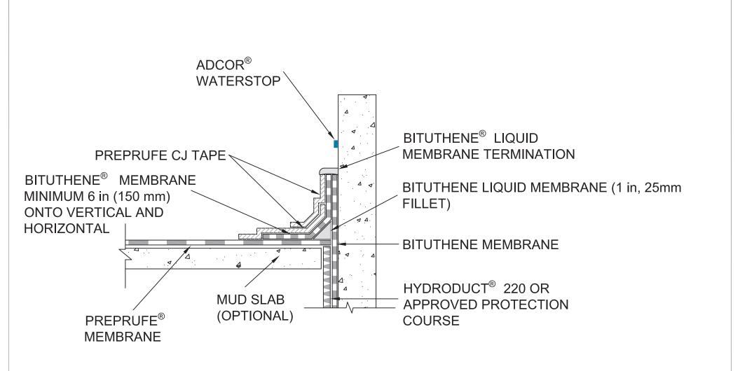
NOTES - IF A MUDSLAB IS NOT USED, THE SUBSTRATE TO ACCEPT THE BITUTHENE LIQUID MEMBRANE MUST BE GROUTED SOLID TO PROVIDE AN ACCEPTABLE SUBSTRATE FOR THE LIQUID MEMBRANE - GCP MAY REQUIRE AN ALTERNATE GCP WATERSTOP BASED ON DESIGN CONDITIONS
