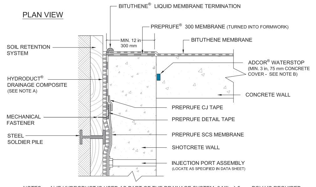
NOTES: A) IF HYDRODUCT IS USED AS PART OF THE DRAINAGE SYSTEM, 6 MIL, 1.5 mm POLY IS REQUIRED BETWEEN THE HYDRODUCT AND THE PREPRUFE SCS MEMBRANE
