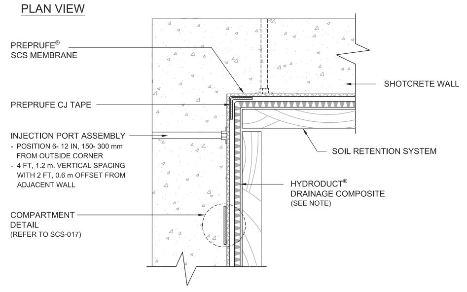
NOTE: IF HYDRODUCT IS USED AS PART OF THE DRAINAGE SYSTEM, 6 MIL, 1.5 mm POLY IS REQUIRED BETWEEN THE HYDRODUCT AND THE PREPRUFE SCS MEMBRANE
