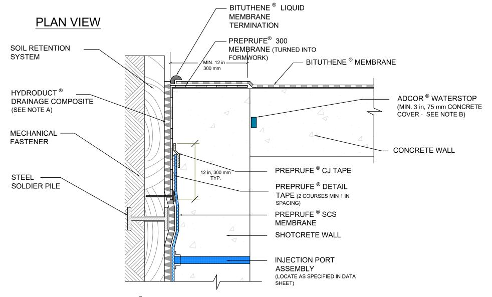
NOTES: A) IF HYDRODUCT <sup>®</sup> IS USED AS PART OF THE DRAINAGE SYSTEM, 6 MIL, 1.5 mm POLY IS REQUIRED BETWEEN THE HYDRODUCT <sup>®</sup> AND THE PREPRUFE <sup>®</sup> SCS MEMBRANE
