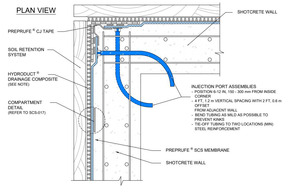
NOTE: IF HYDRODUCT IS USED AS PART OF THE DRAINAGE SYSTEM, 6 MIL,1.5 mm POLY IS REQUIRED BETWEEN HYDRODUCT AND PREPRUFE SCS MEMBRANE
