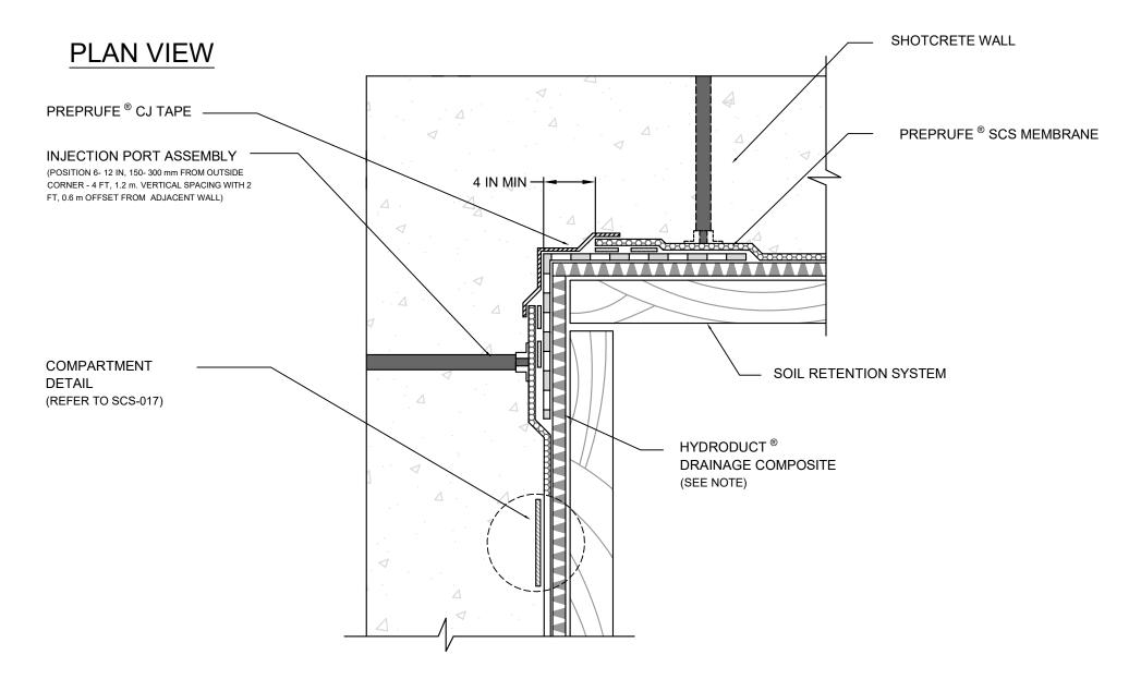
NOTE: IF HYDRODUCT <sup>®</sup> IS USED AS PART OF THE DRAINAGE SYSTEM, 6 MIL, 1.5 mm POLY IS REQUIRED BETWEEN THE HYDRODUCT <sup>®</sup> AND THE PREPRUFE <sup>®</sup> SCS MEMBRANE
