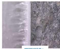
Figure 4. Continuous Adhesive Bond between PREPRUFE ® Plus and concrete
